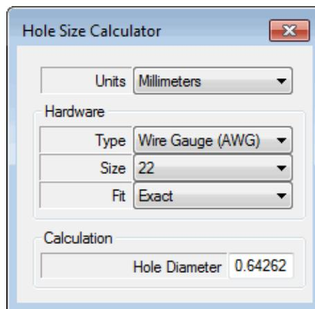
The screenshot shows a dialog box titled "Hole Size Calculator". It has a close button in the top right corner. The dialog is organized into sections: "Units" with a dropdown menu set to "Millimeters"; "Hardware" which contains three dropdown menus: "Type" set to "Wire Gauge (AWG)", "Size" set to "22", and "Fit" set to "Exact"; and "Calculation" which has a text field labeled "Hole Diameter" containing the value "0.64262".
