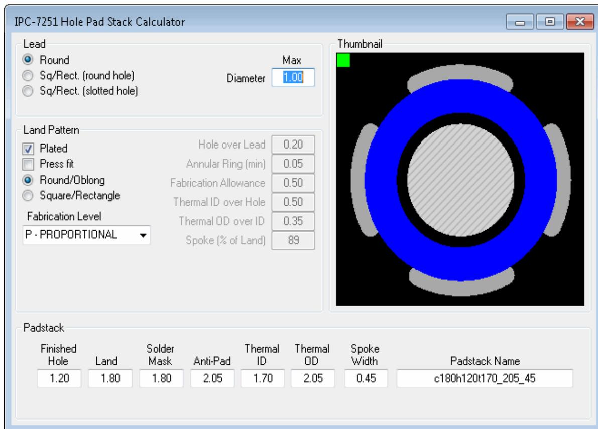
This calculator is similar to the Hole Size Calculator to the extent that the hole size can be calculated based on the size and shape of the object that the hole will accommodate and the fabrication level of the application. Additionally the hole size can be directly specified.
