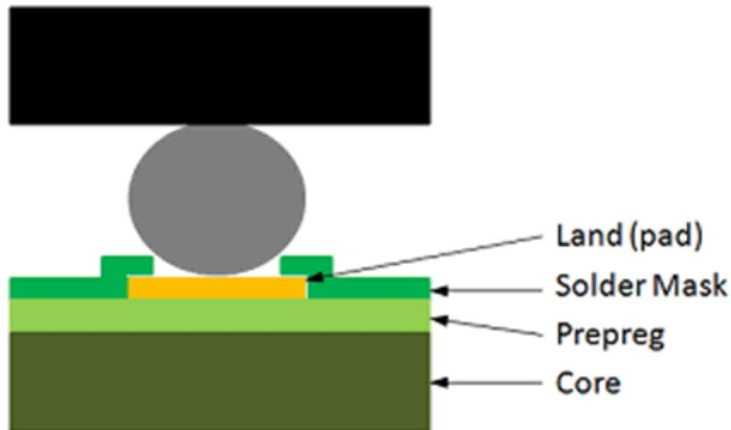
Solder mask defined lands are also used for Flexible circuit boards for the same reason, to hold the land (pad) to the PCB surface to prevent the land from ripping away from the PCB material. When you use solder mask defined lands you must indicate which parts deviate from the 1:1 scale solder mask rule in the fabrication drawing notes to notify the CAM operator not to swell these solder mask features.
